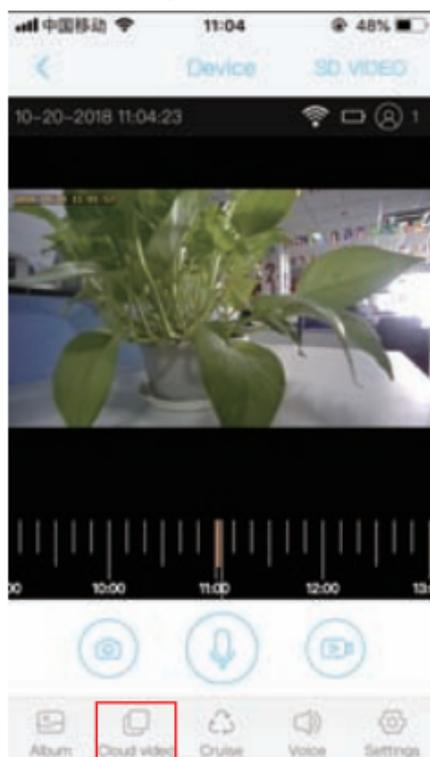
3). Cloud Storage Description: When the device is in sleep state, PIR trigger or press the doorbell button, the device will automatically upload 8 seconds of video to the cloud, each device can record 20 events per day, and have a week of permanent free storage cloud for users to use.
